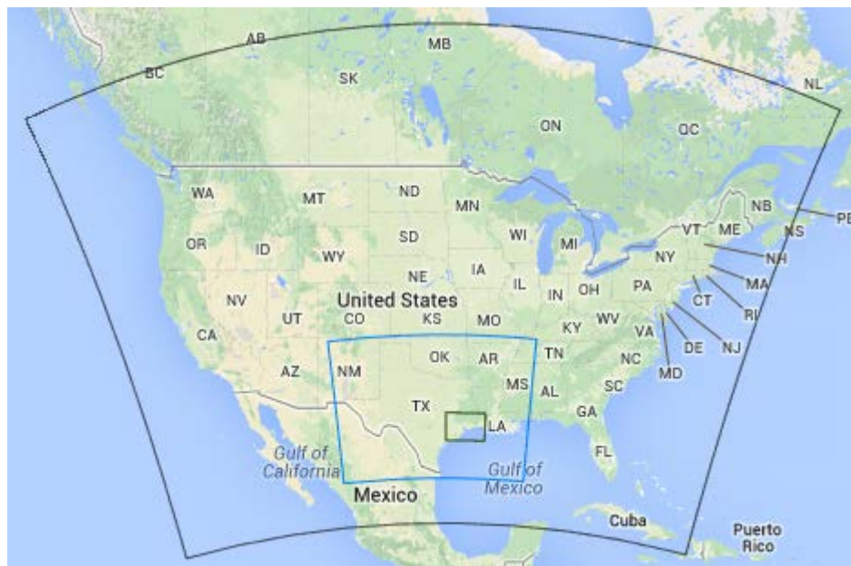
Figure 14. CAMx modeling domain with outer 36 km grid and nest 12 km (blue) and 4 km (green) grids
